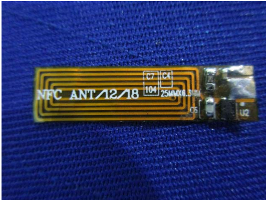
EUT – NFC Board Top View
