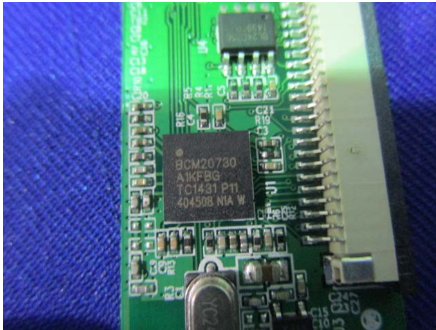
EUT –RF Chip View
