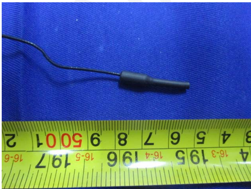
EUT –RF Antenna View
