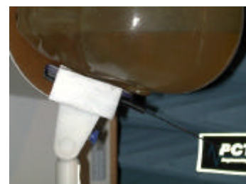
Figure 14. Head SAR Test Setup
