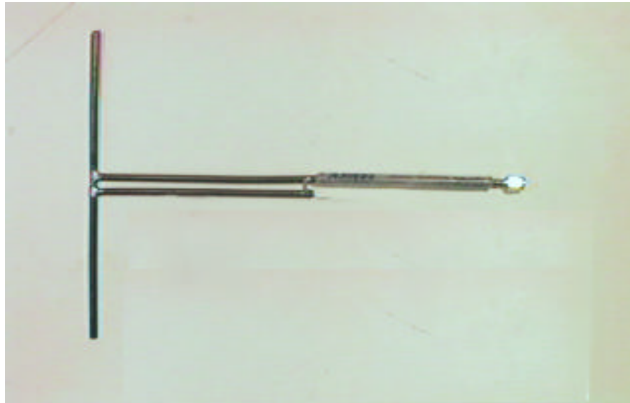
Reference Dipole Antenna Used for ERP Measurement
