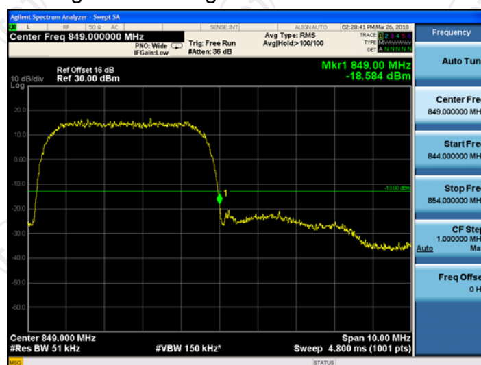
Higher Band Edge Plot on Channel 4233
