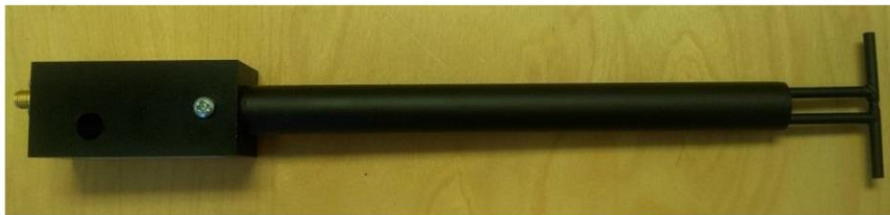
Figure 1 – MVG COMOSAR Validation Dipole
