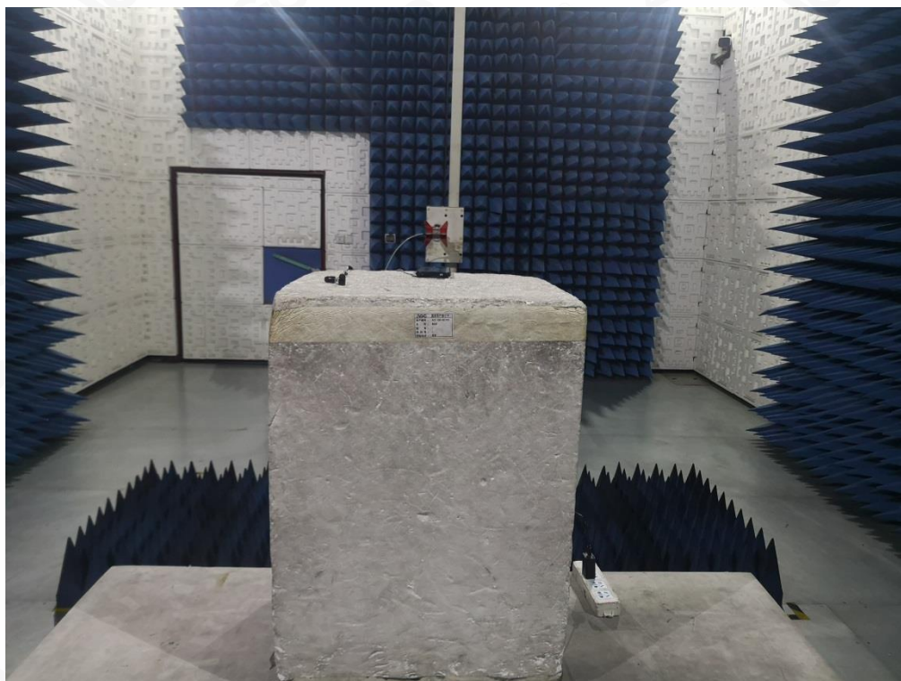
FCC RADIATED EMISSION TEST SETUP ABOVE 1GHZ
