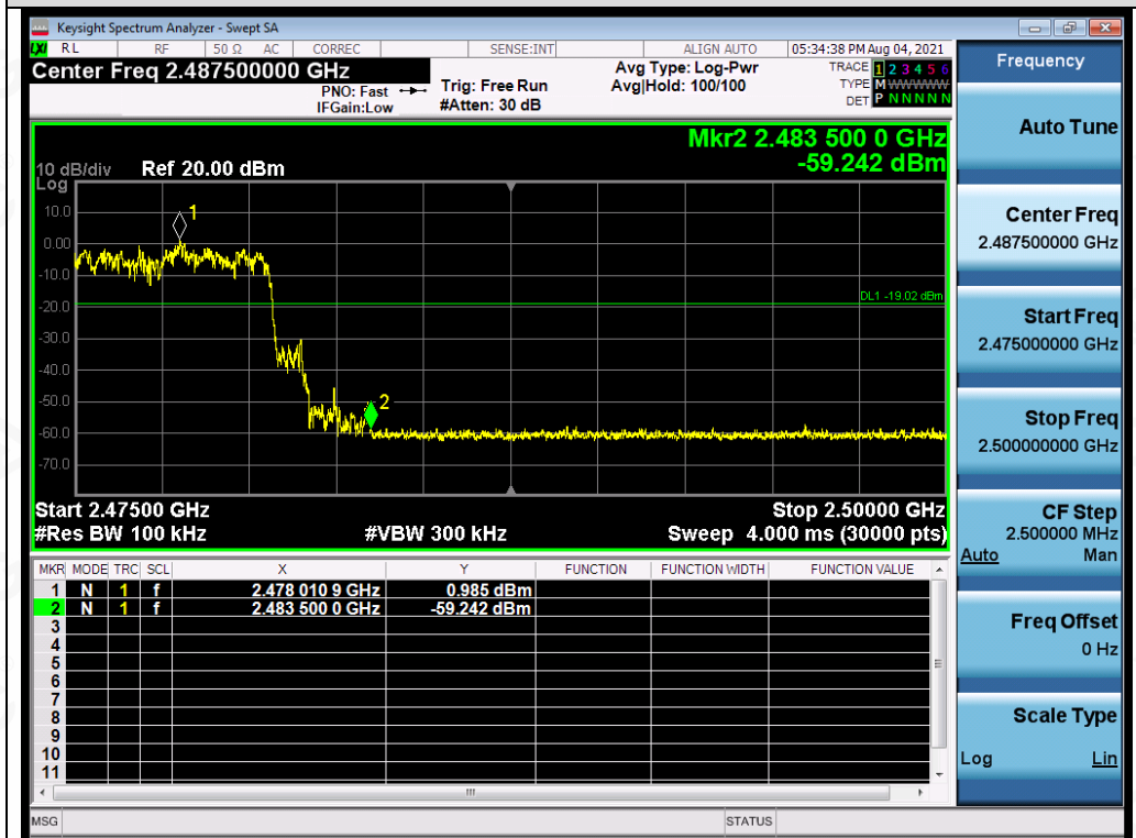
Test_Graph_EDR_HOP_ANT1_NA_3Mbps_Higher Band Edge Emissions
