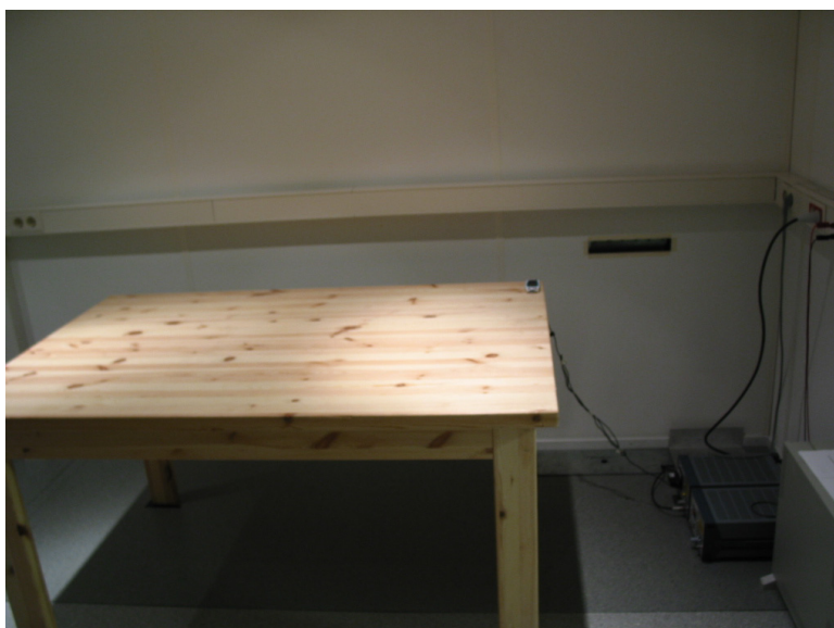
Picture 1. AC conducted emission measurement setup
