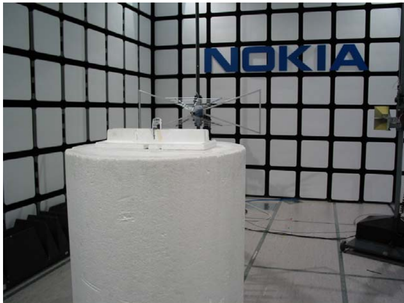
RF Output power measurement
