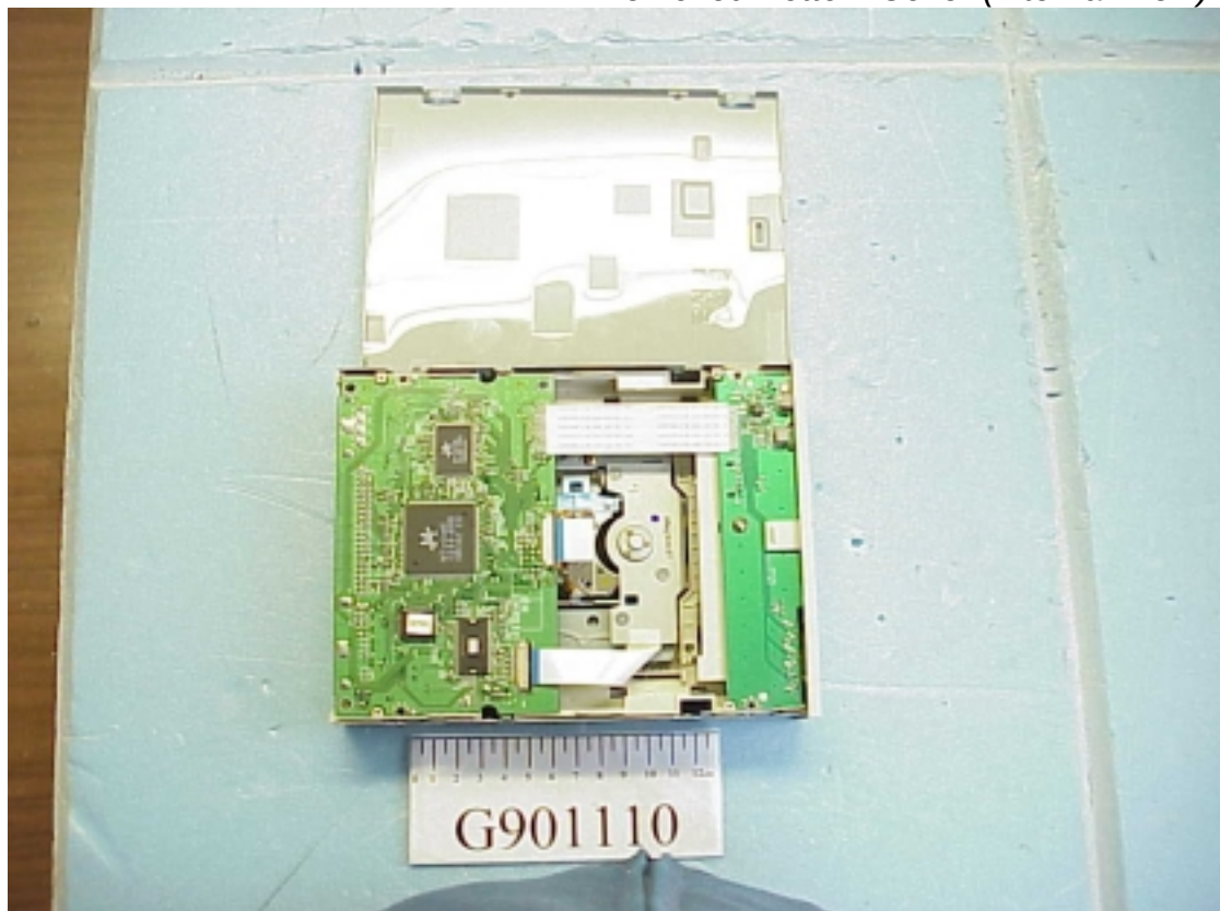
Figure 4 Removed Mother Board & Control Board (Internal View)
