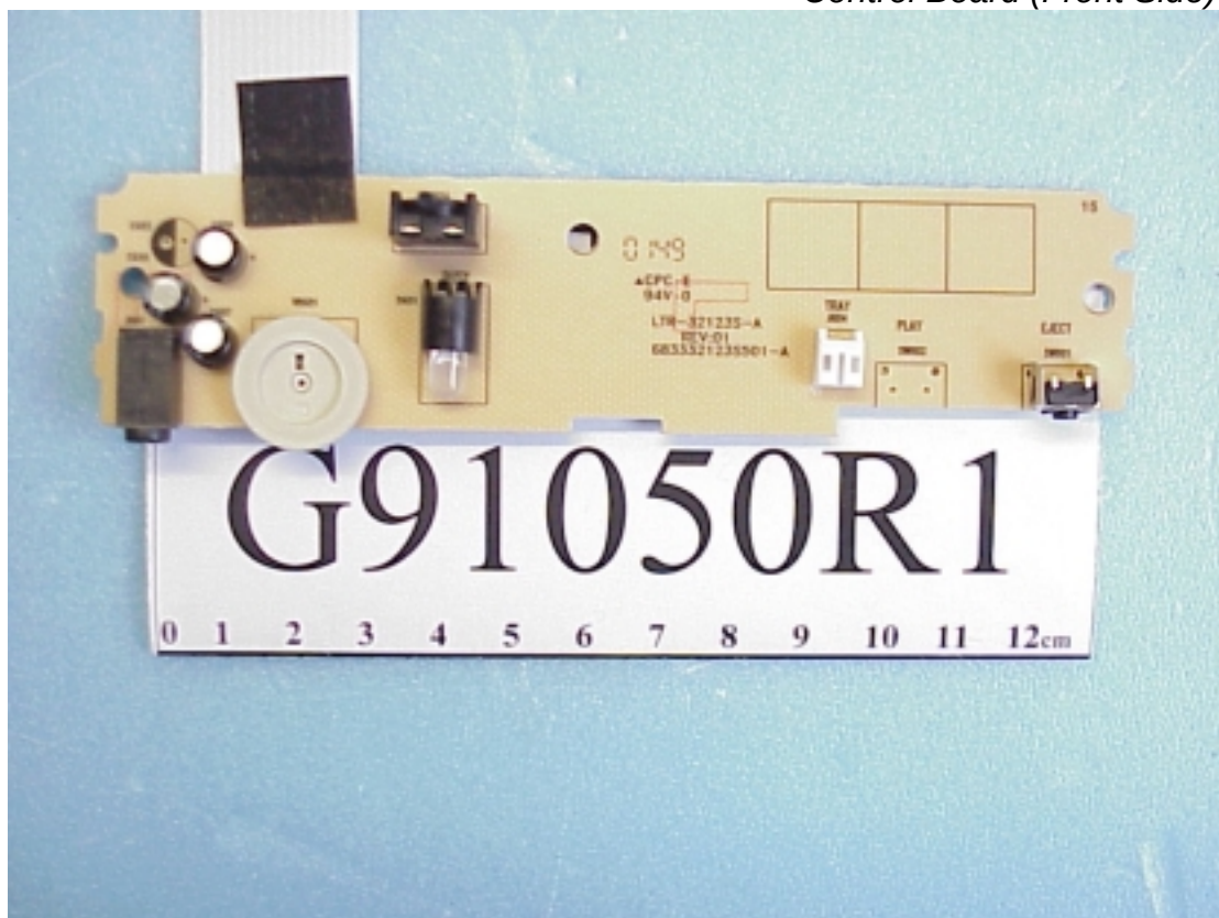
Figure 19 Control Board (Front Side)
