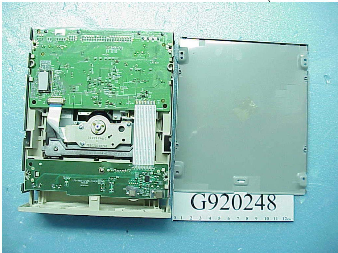
Figure 5 CD-R/RW DRIVE Internal View (Removed Bottom Case)
