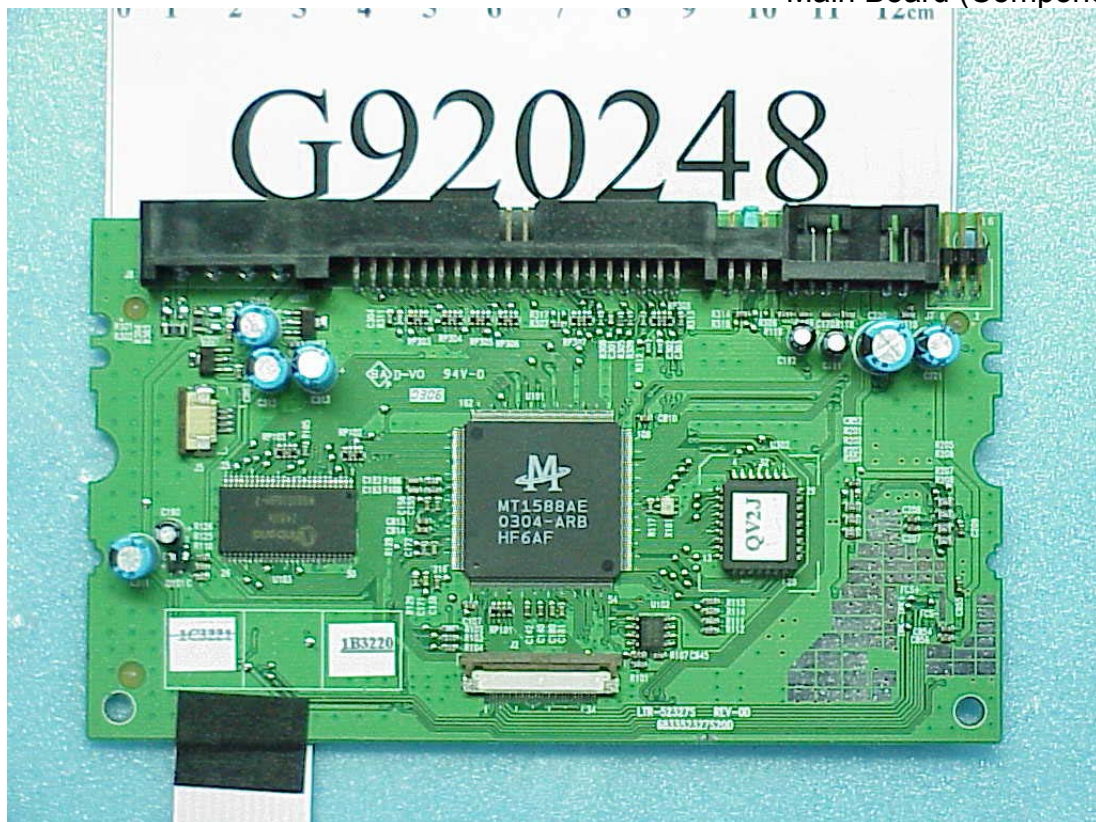
Figure 7 CD-R/RW DRIVE Main Board (Component Side)
