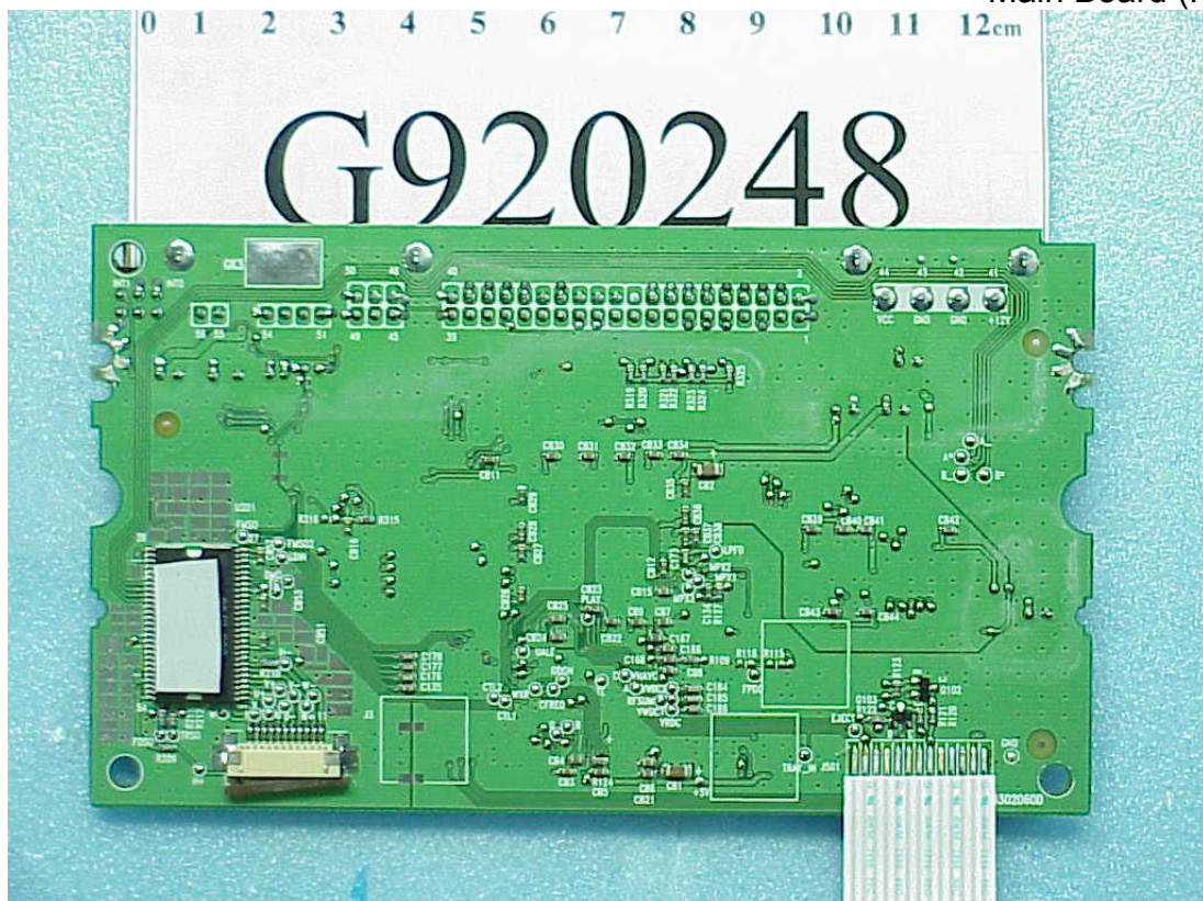
Figure 8 CD-R/RW DRIVE Main Board (Foil Side)
