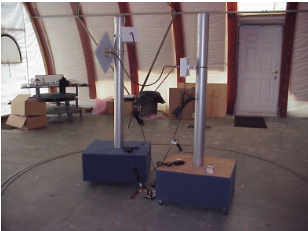
Flat Panel Point-to-Multipoint 23 dBi Gain
