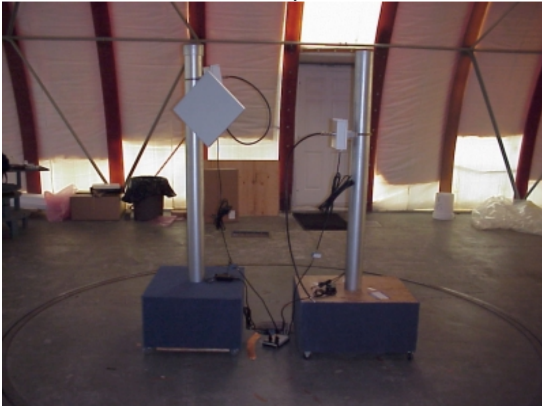
Flat Panel Point-to-Multipoint 23 dBi Gain
