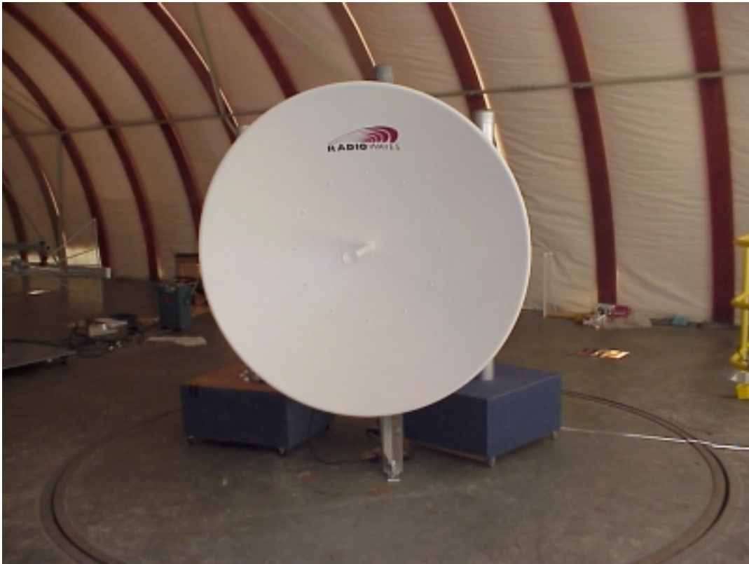
6' Parabolic Point-to-Point 37.6 dBi Gain
