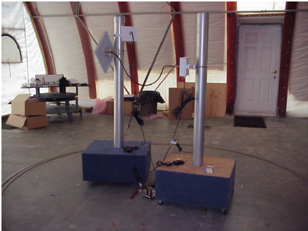
Flat Panel Point-to-Multipoint 23 dBi Gain
