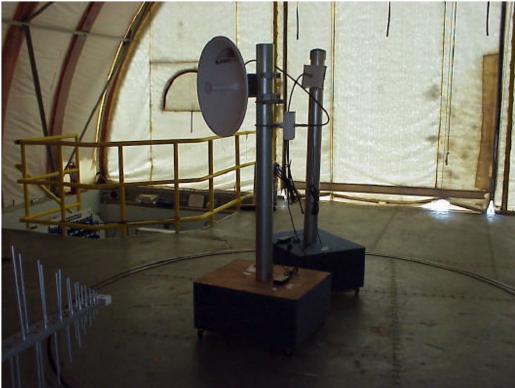
2' Parabolic Point-to-Point 28 dBi Gain
