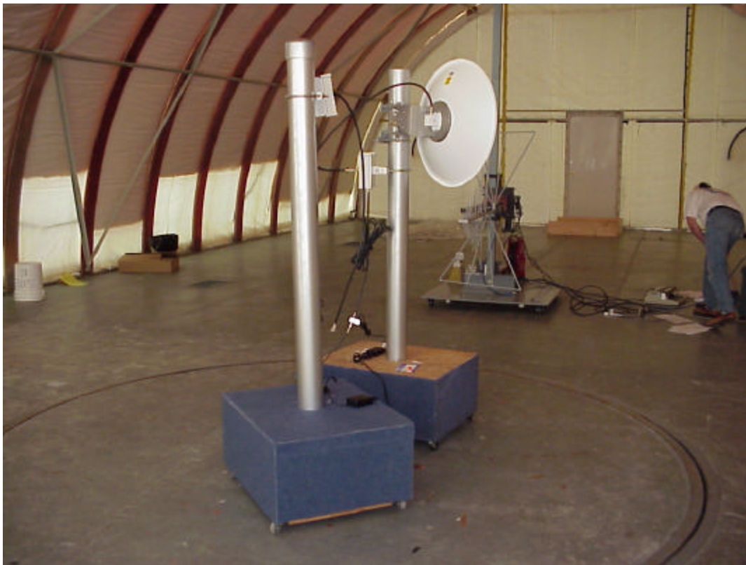
6' Parabolic Point-to-Point 37.6 dBi Gain
