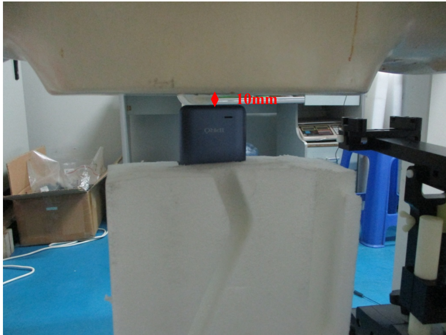
Body Bottom Setup Photo(10mm)
