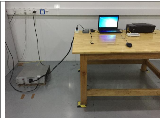
Conducted Emissions Test Setup – Front View
