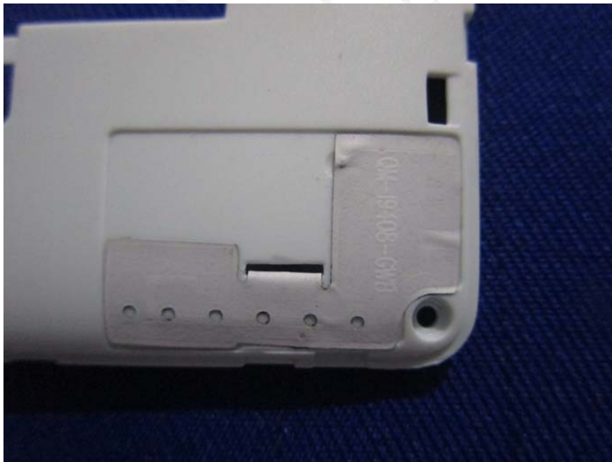
EUT -BT & Wifi & GPS Antenna View
