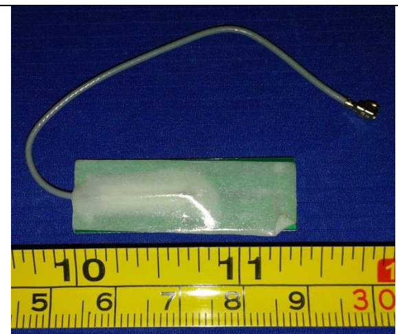
Laird antenna - P/N (453564252521r1444) Bottom View
