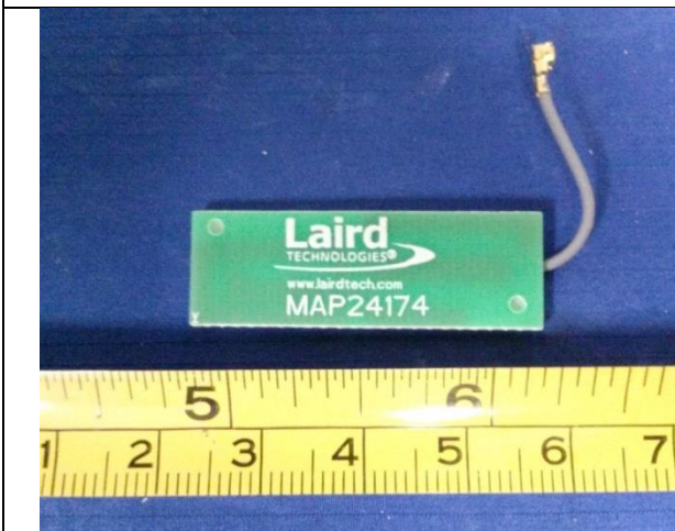
Laird antenna - P/N (453564553001r1444) Top View
