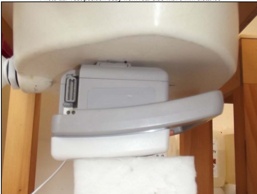
Photo 12: Test position body worn rear side with 0 mm distance
