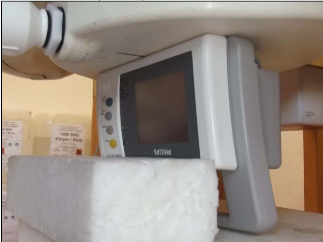
Photo 13: Test position body worn bottom side with 0 mm distance
