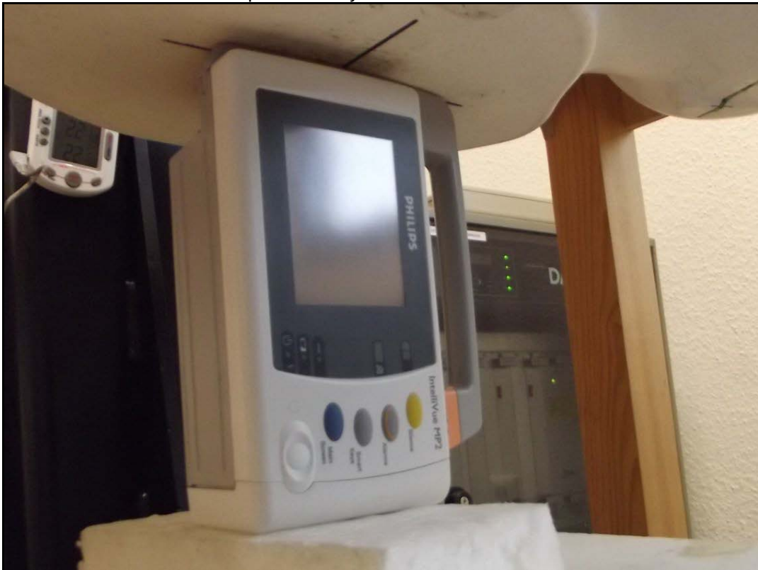
Photo 14: Test position body worn left side with 0 mm distance
