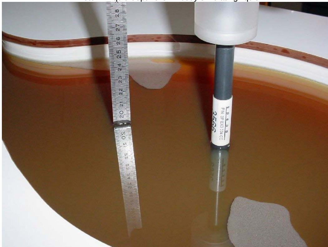
Photo 2: Liquid depth 5 GHz body simulating liquid
