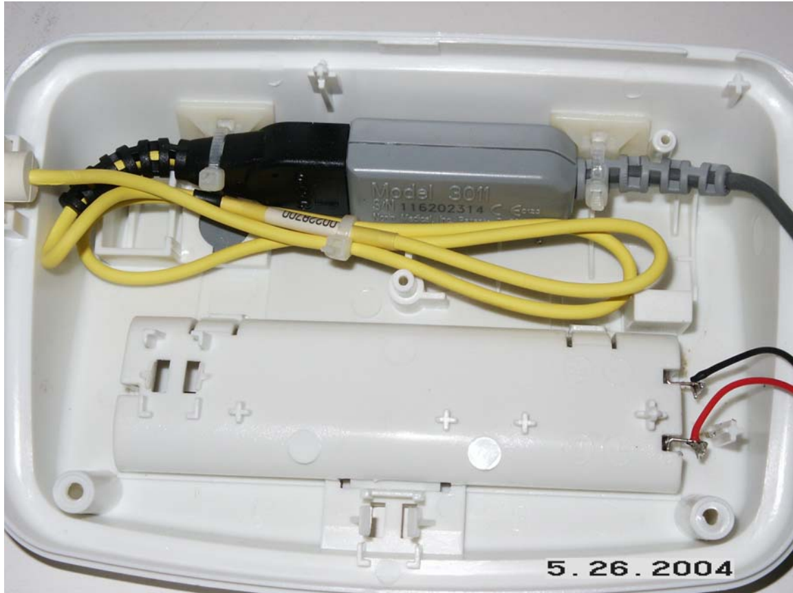
Inside of housing with PCB removed showing the SPO2 measurement device and battery connections.
