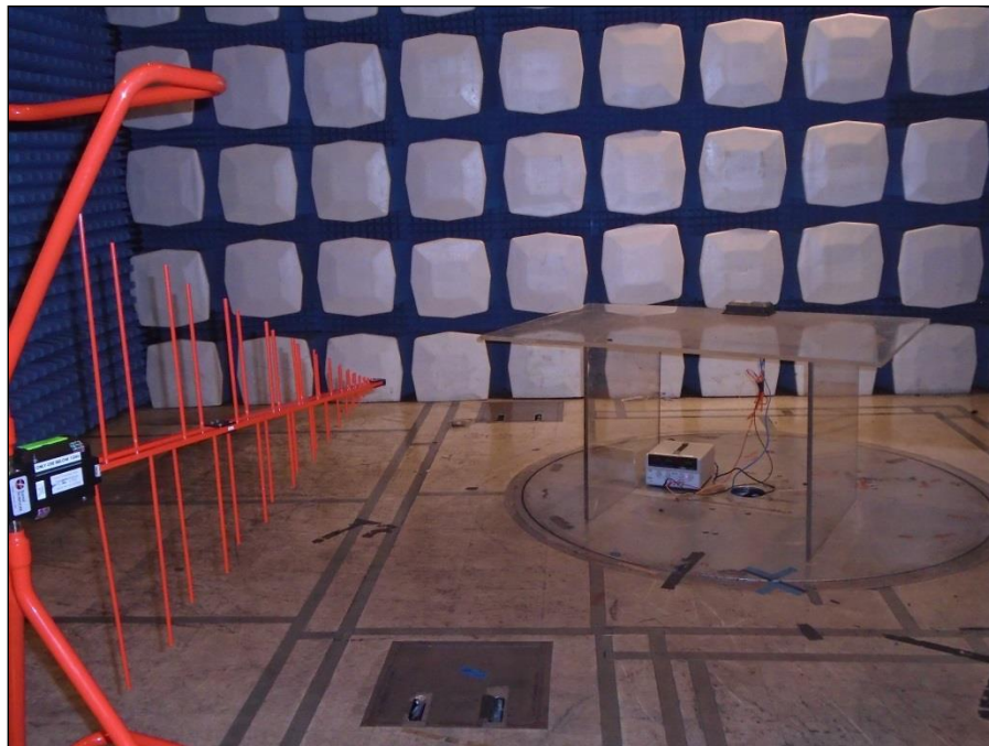
Photograph 2. Spurious Radiated Emissions, upto 1 GHz Test Setup
