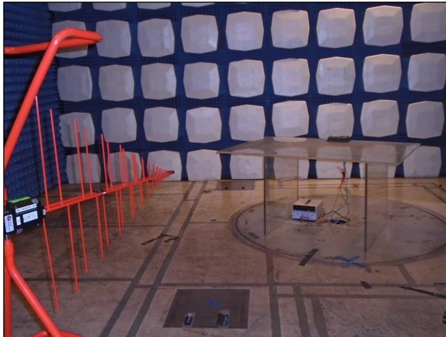
Photograph 1. Radiated Spurious Emissions, Test Setup, 30 MHz – 1 GHz
