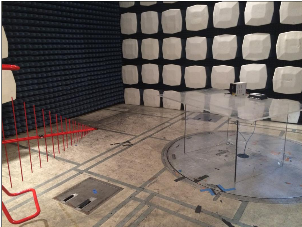
Photograph 1. Radiated Emission, Set up Below 1 GHz, Test Results
