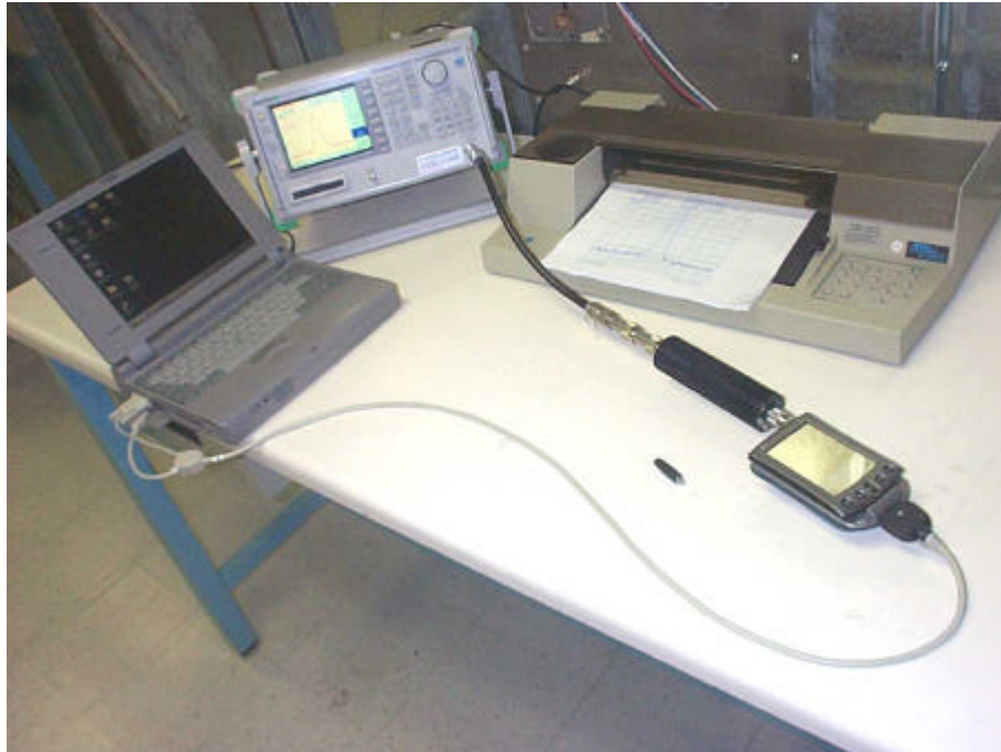
Testing Spurious Radiation from Transmitter at Antenna Port Palm attached to DUALWAVE M Wireless Modem and connected to PC
