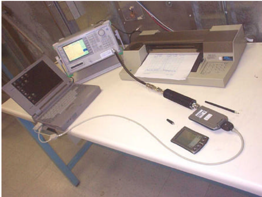
Testing Spurious Radiation from Transmitter at Antenna Port on DUALWAVE M Wireless Modem only connected to PC
