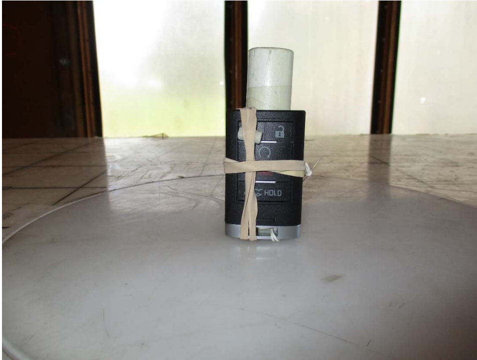
Test Setup, X Axis, Below 1 GHz
