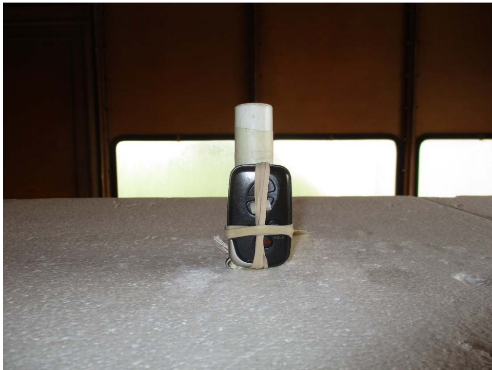
Test Setup, X Axis, Above 1 GHz
