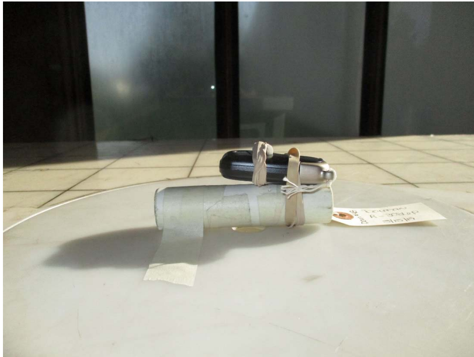
Test Setup, Z Axis, Below 1 GHz
