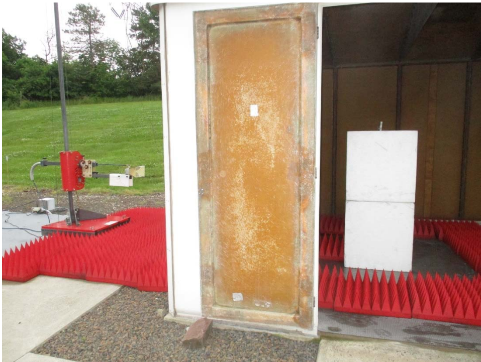
Vertical Antenna Polarization, Above 1 GHz
