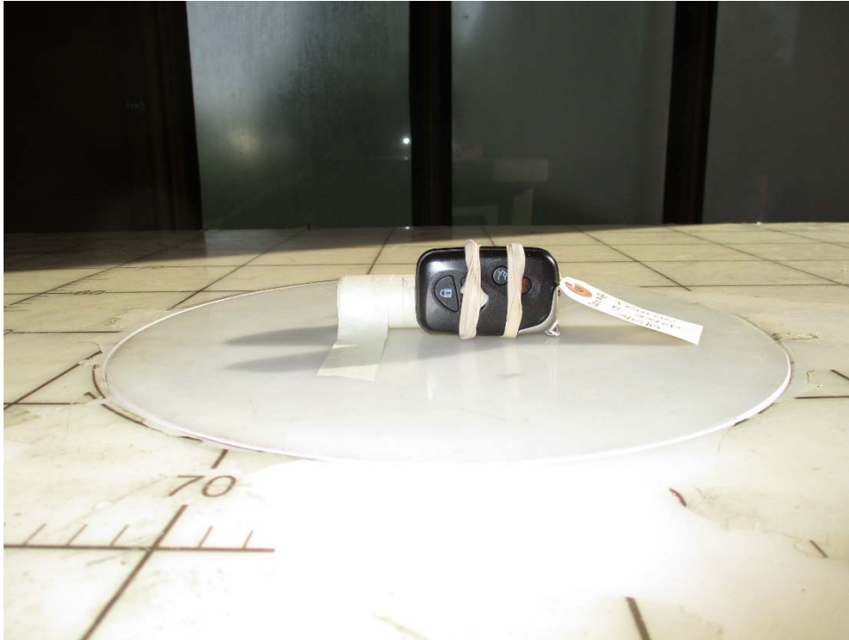
Test Setup, Y Axis, Below 1 GHz
