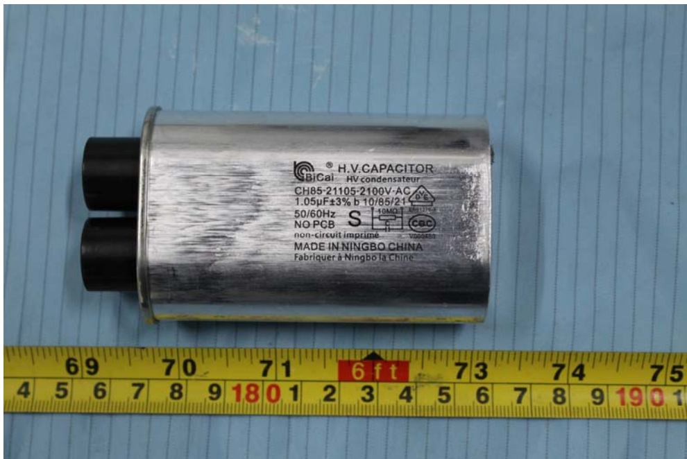
EUT –High Voltage Capacitor View
