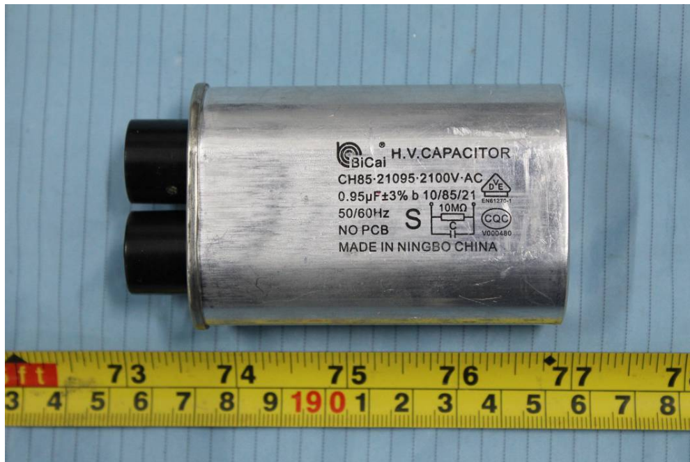
EUT –High Voltage Capacitor View
