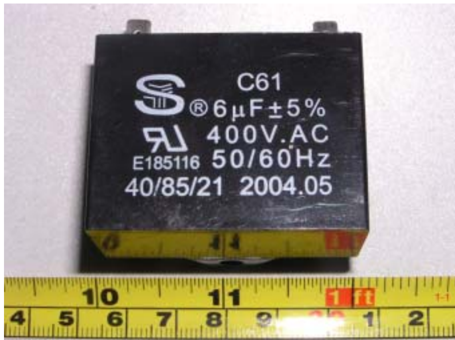
EUT – Filter Capacitor 1 View
