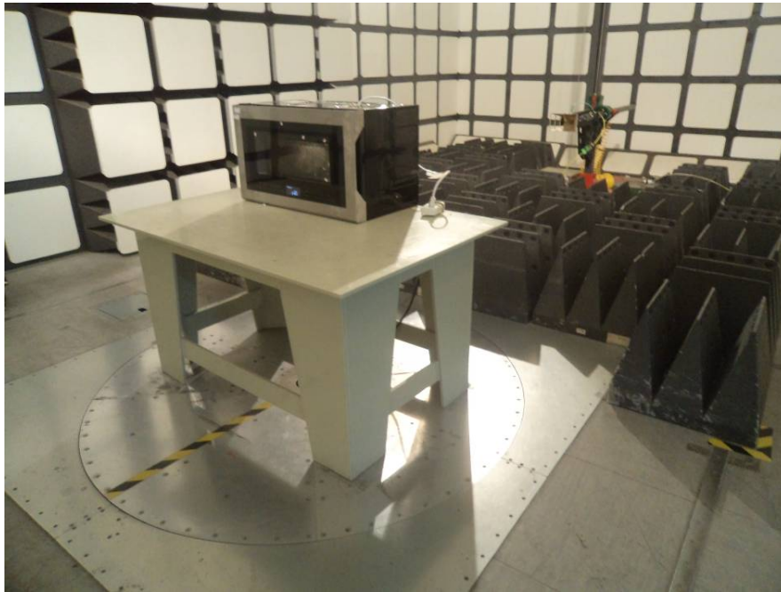
Radiated Emissions - Front View (Above 1 GHz)
