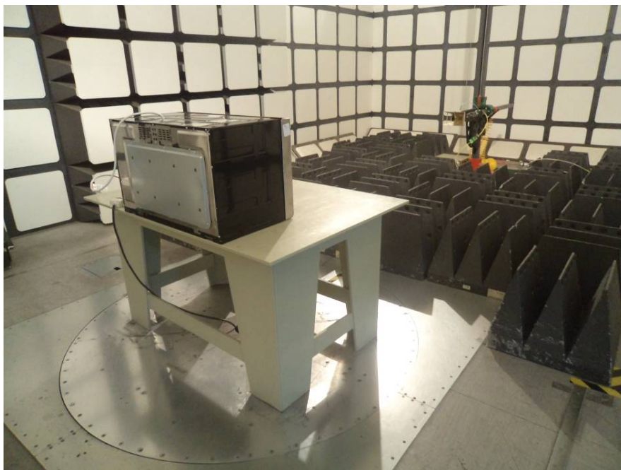
Radiated Emissions - Rear View (Above 1 GHz)
