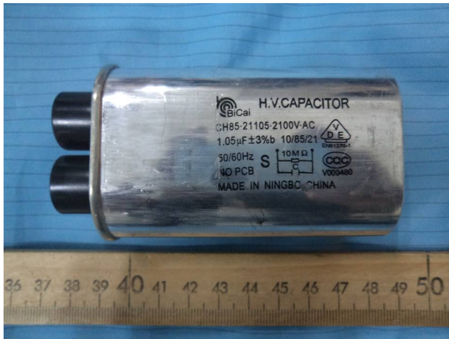
EUT – H.V. Capacitor View
