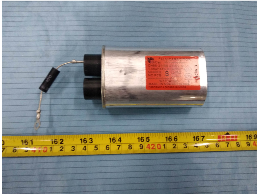
EUT – H.V. Capacitor Top View
