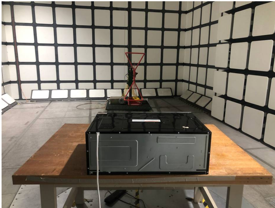
Radiated Emissions - Rear View (30 MHz – 1 GHz)
