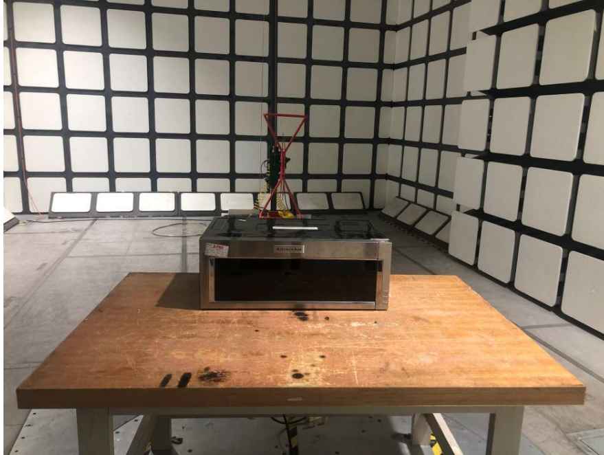
Radiated Emissions - Front View (30 MHz – 1 GHz)
