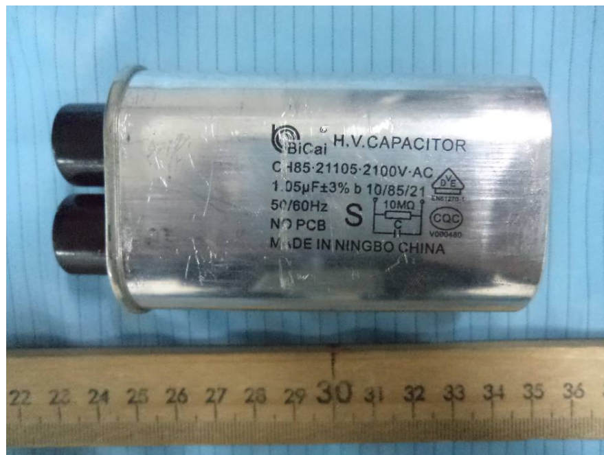
EUT – H.V. Capacitor View
