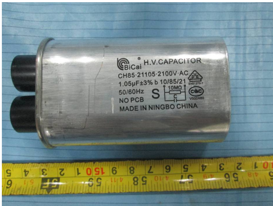
EUT – H.V. Capacitor View
