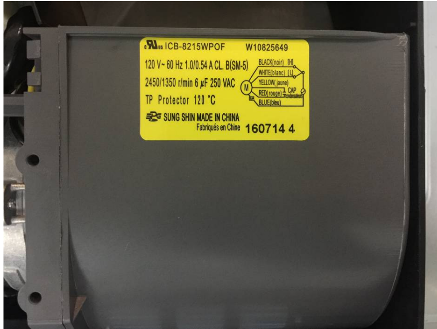
EUT – Fans Label View
