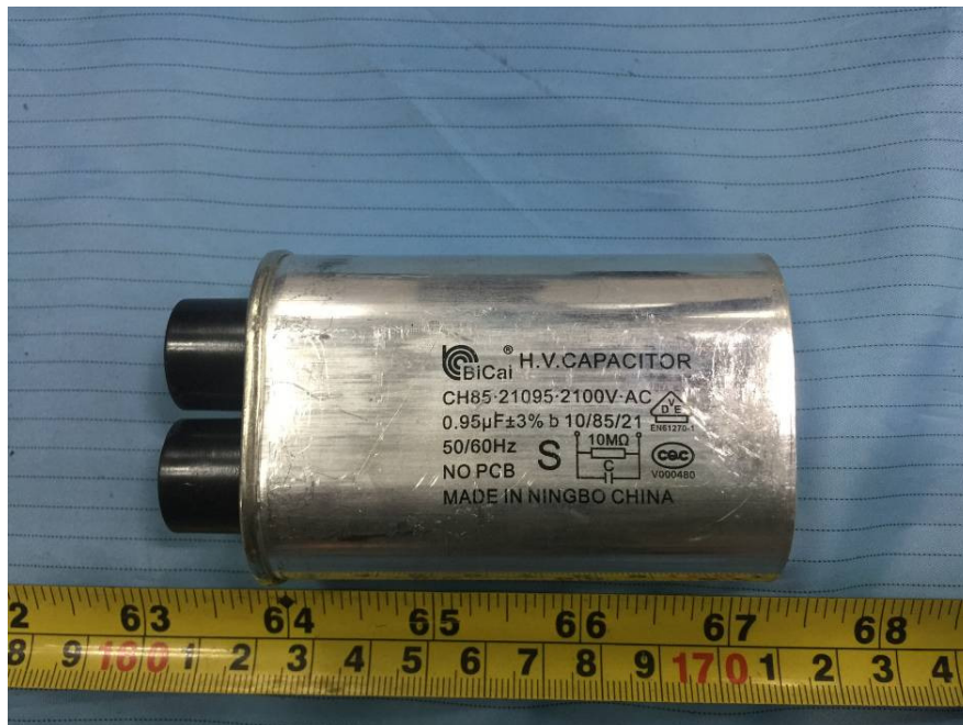
EUT –H.V. CAPACTOR View
