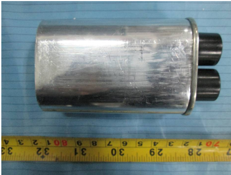
EUT – H.V. Capacitor Bottom View
