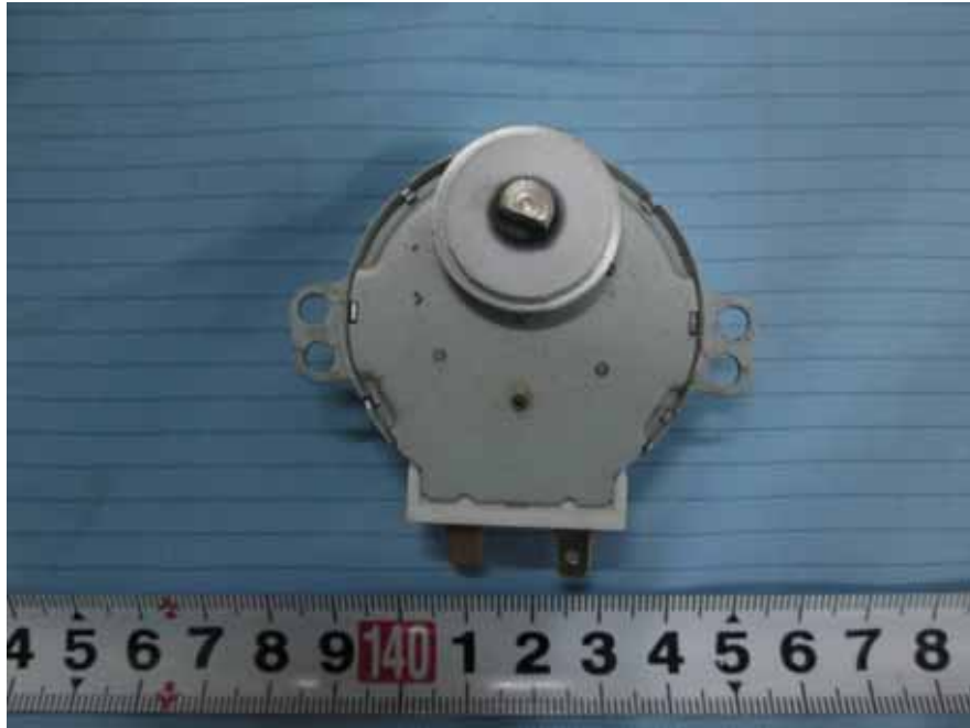
EUT – Motor Bottom View
