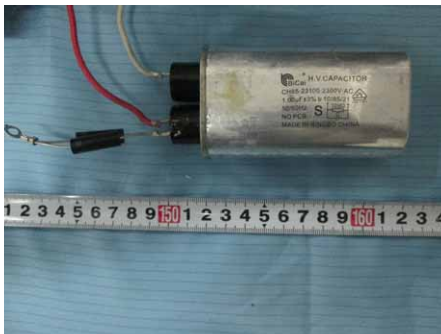
EUT – H.V. Capacitor Front View
