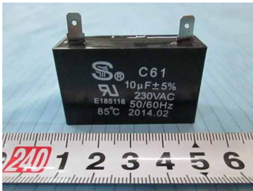
EUT – C61 Capacitor View
