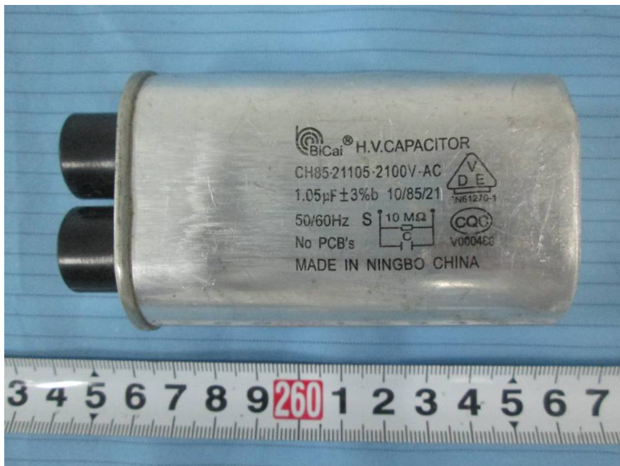
EUT – H.V. Capacitor View
