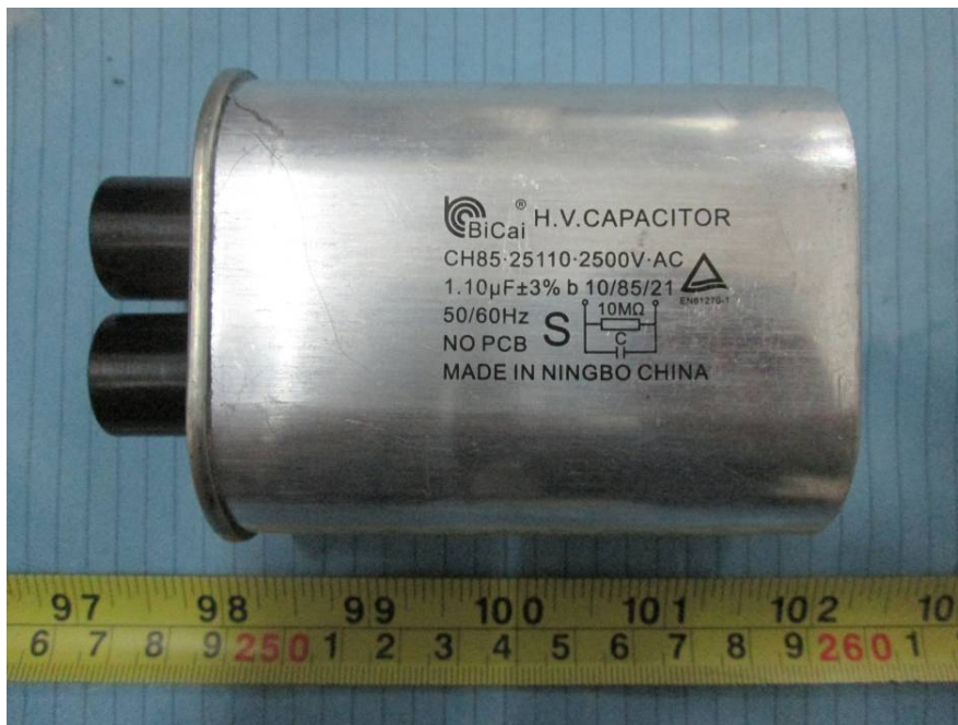
EUT – H.V. Capacitor View
