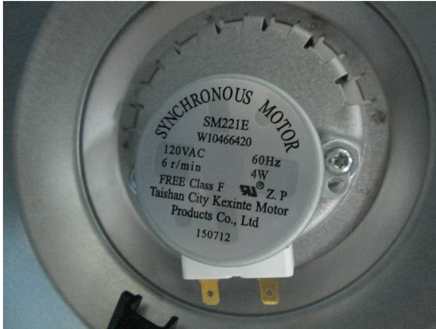
EUT – Motor 2 Label View
