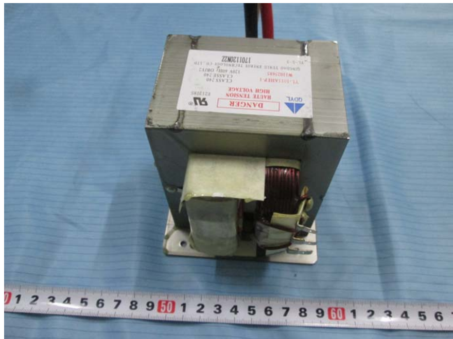
EUT – Transformer View
