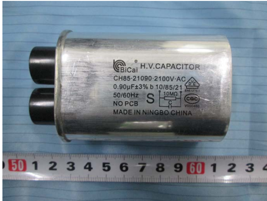
EUT –H.V. CAPACITOR View
