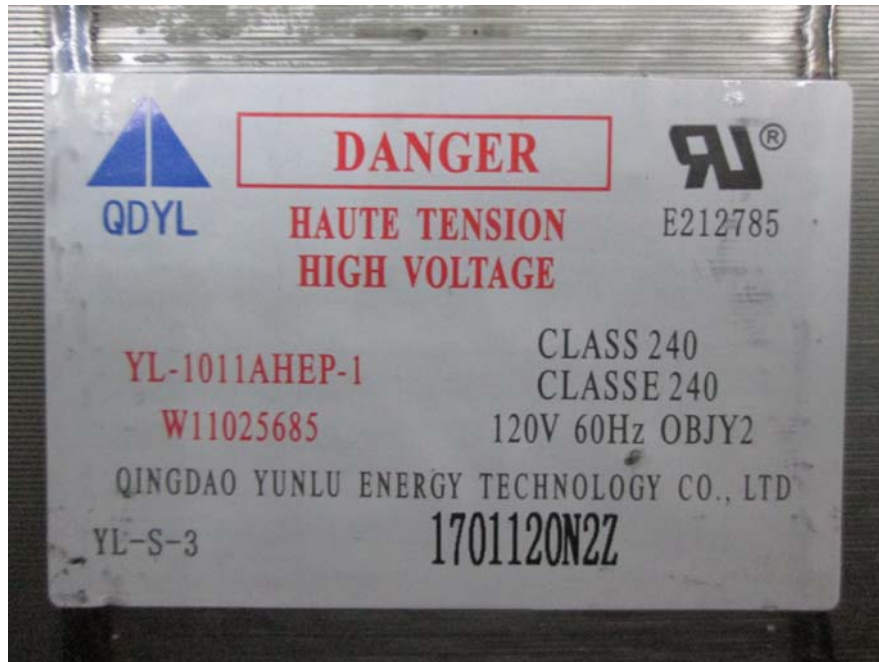
EUT – Transformer Label View
