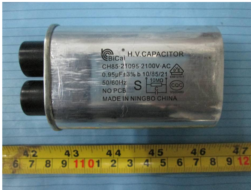
EUT – H.V. Capacitor Front View
