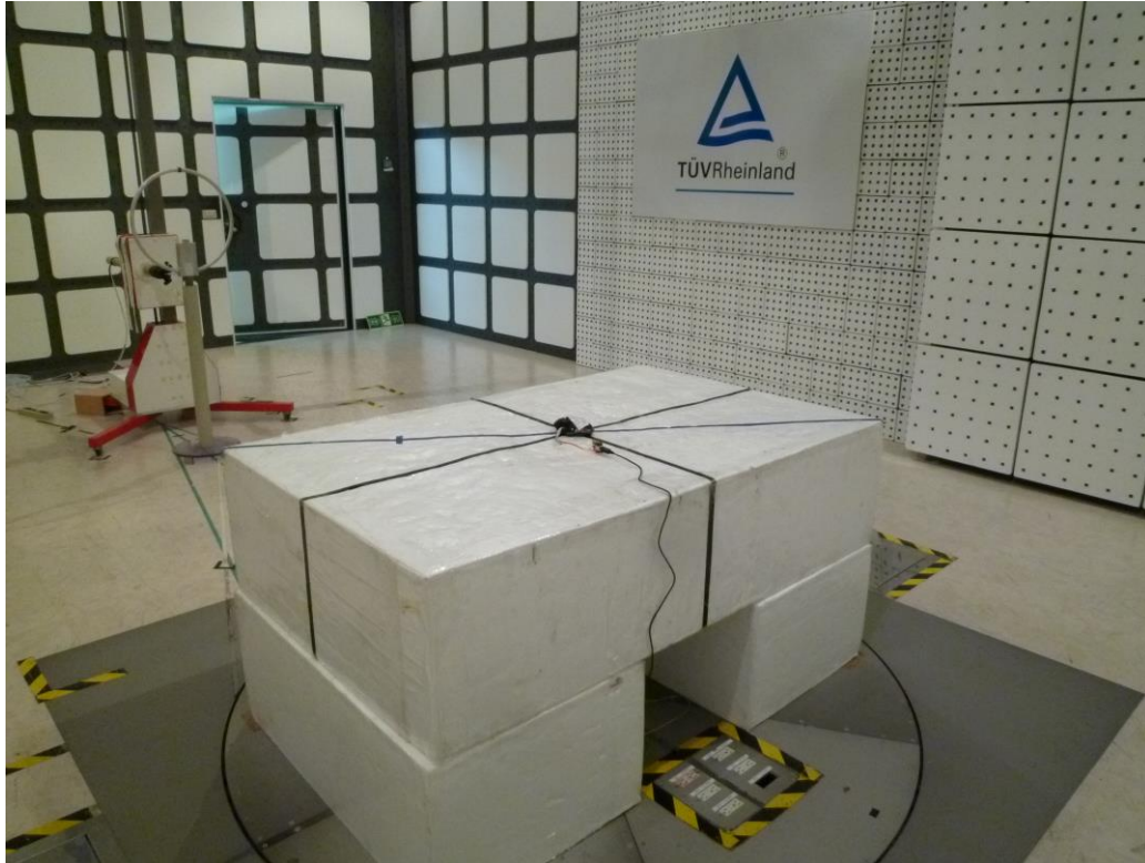
Photograph 4: Set-up for Spurious Emissions (Back View 3)
