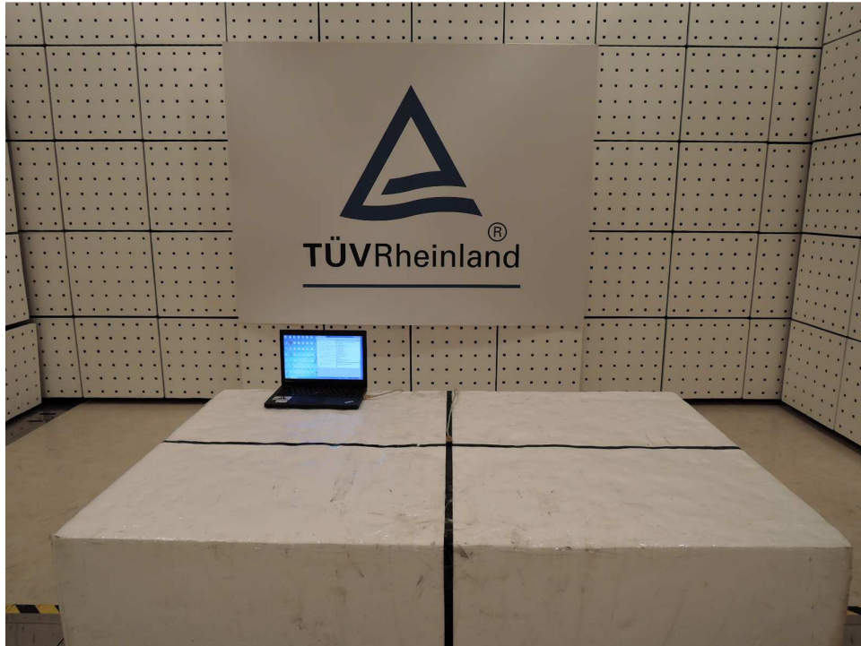
Photograph 1: Set-up for Spurious Emissions (Front View)
