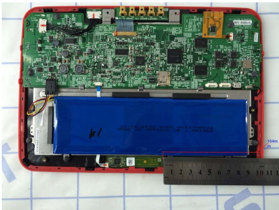
Antenna separation distance view-2
