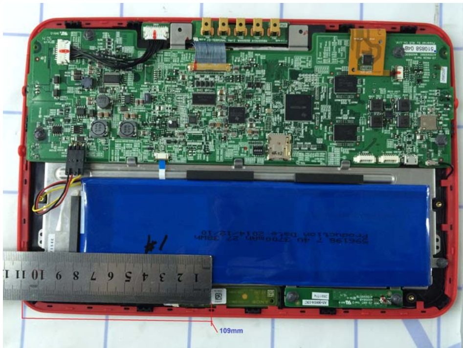
Antenna separation distance view-4
