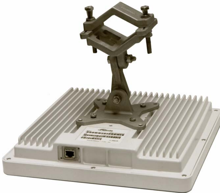
Figure 4-4 Alternate ODU Mounting Bracket
