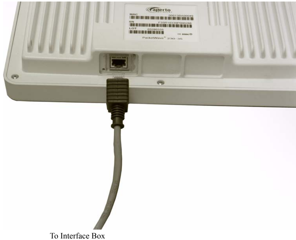
Figure 4-7 Connection to the Outdoor Unit
