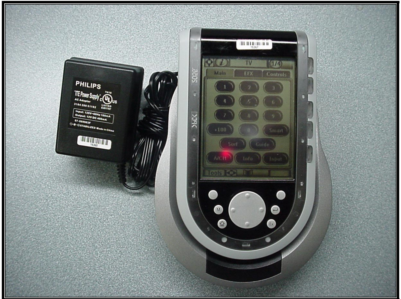
PHOTOGRAPH 7: TOUCH SCREEN REMOTE CONTROL IN DOCKING STATION
