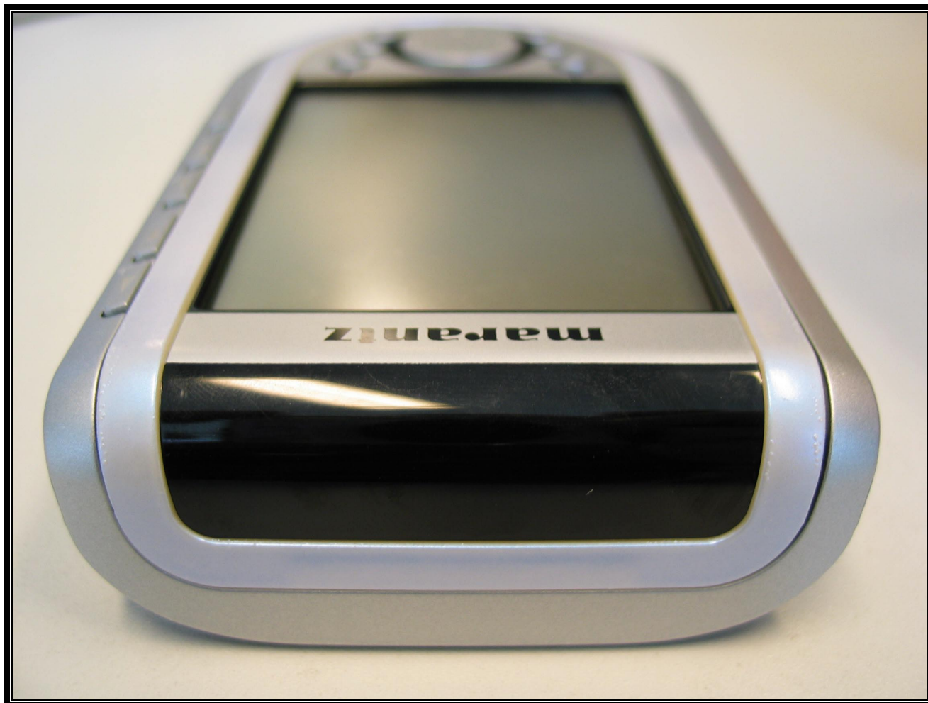
PHOTOGRAPH 13: IR WINDOW VIEW
